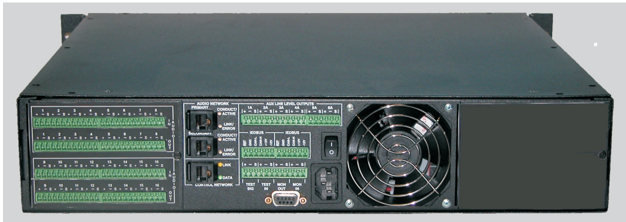
Figure 2 - T9116 Digital Signal Processing Mainframe Rear View
