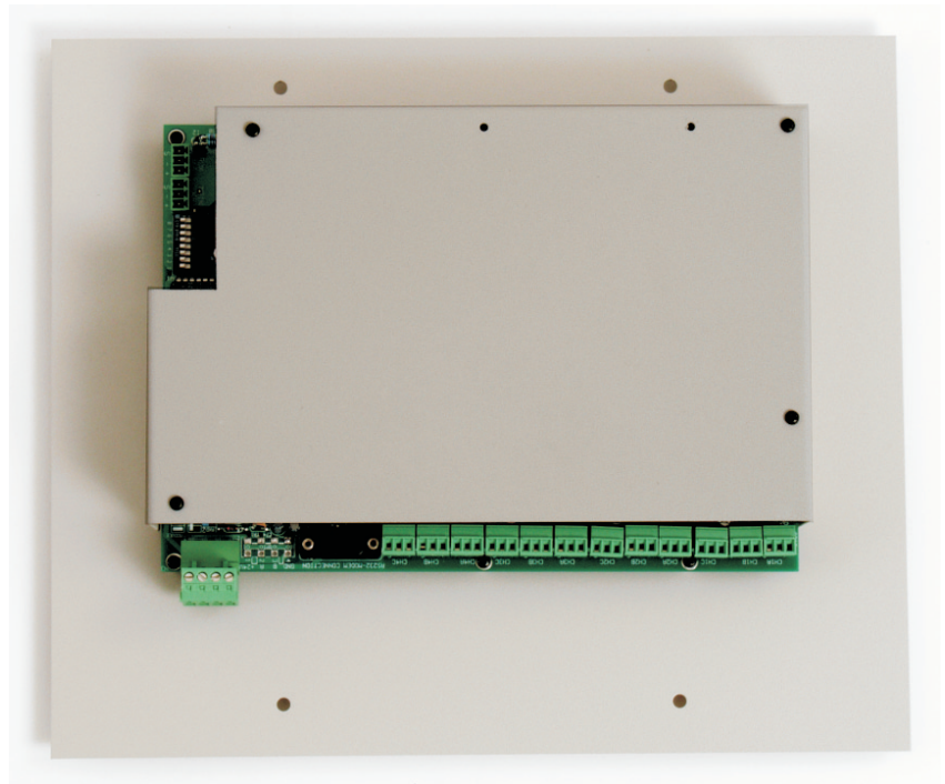
4000RCM Remote Controlled Mixer Wall Mount Version, Rear View showing connectors
