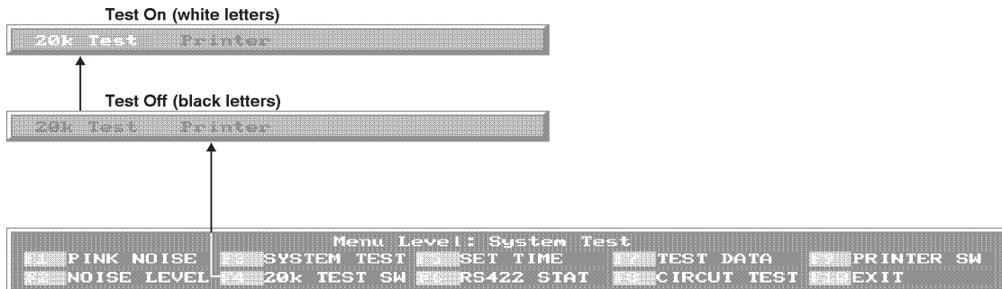
Figure 23 - System Test Menu 20 kHz Test Switch
