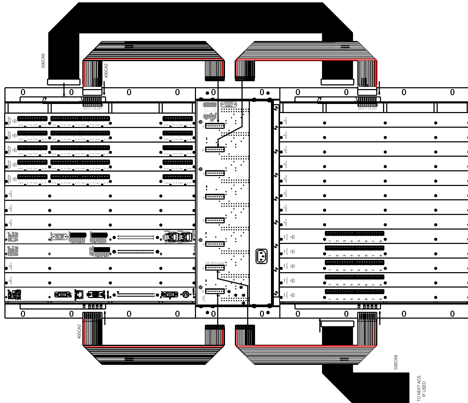
Figure 4 - Typical Power and Multibus Cable Interface For Multiframe ACS Systems with 510CPU, Rear View
